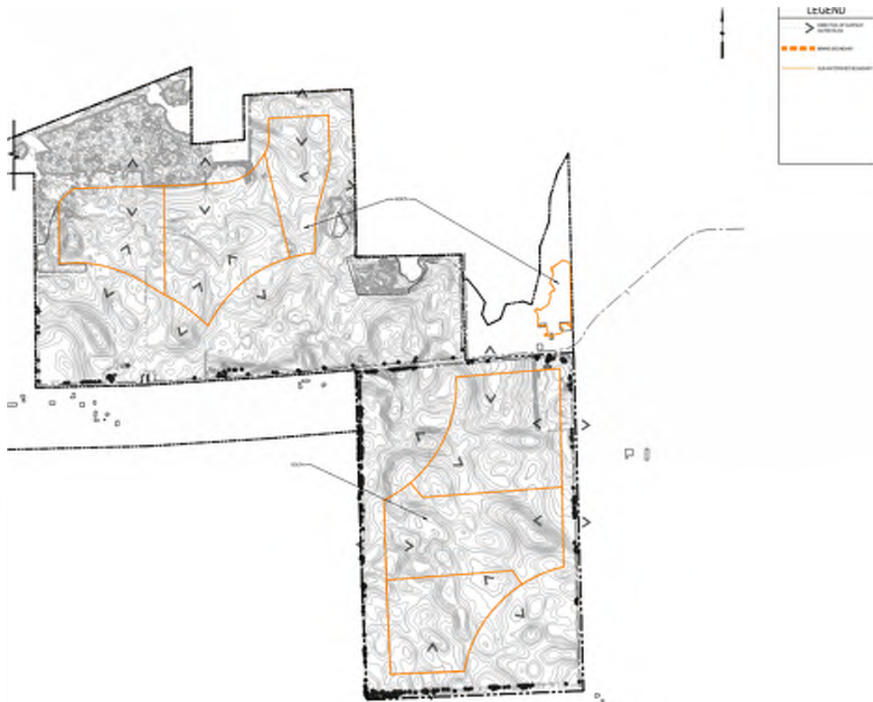
Figure 13 - Existing Drainage Areas
